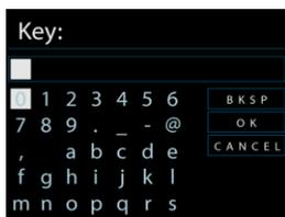
To enter the network's key, use the reel or direction keys on the remote control to move the cursor through the characters and press **OK** (SCAN) to confirm. As each character is selected, the key is built up near the top of the display.
