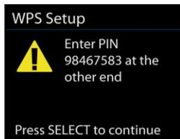
The device generates an 8-digit code number which you enter into the wireless router, access point, or an external registrar.
