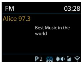
To find a station, press **OK** <sup>(SCAN)</sup>. The frequency display starts to run up as the device scans the FM band. Alternatively, you can scan up or down by pressing and holding the buttons **▼/TUNING-** or **▲/TUNING+** or tune manually with quick presses, or by turning the reel.
