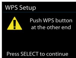
The device prompts you to press the connect button on the router. It then scans for a ready Push Button Connect network and connects.
